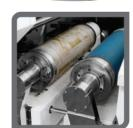
The blanket sleeve is a similar metal construction to the plate sleeve, with bearer size matching and design which reduces blanket wear.
